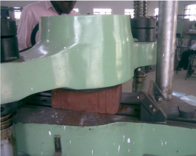
Fig 4. Photograph showing the test setup for brick compressive strength in Universal testing machine
