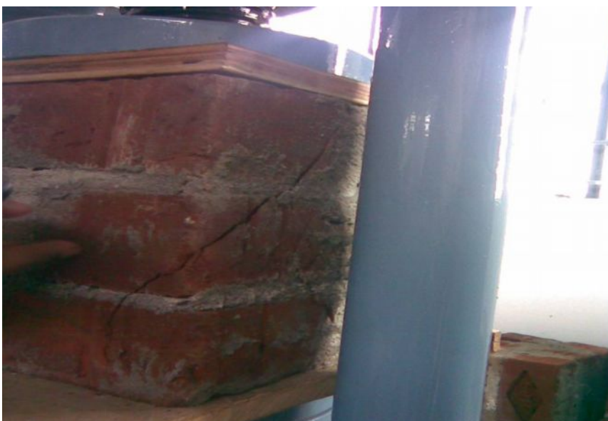
Fig 19. Crack formation in the brick prism during compression in compression testing machine
