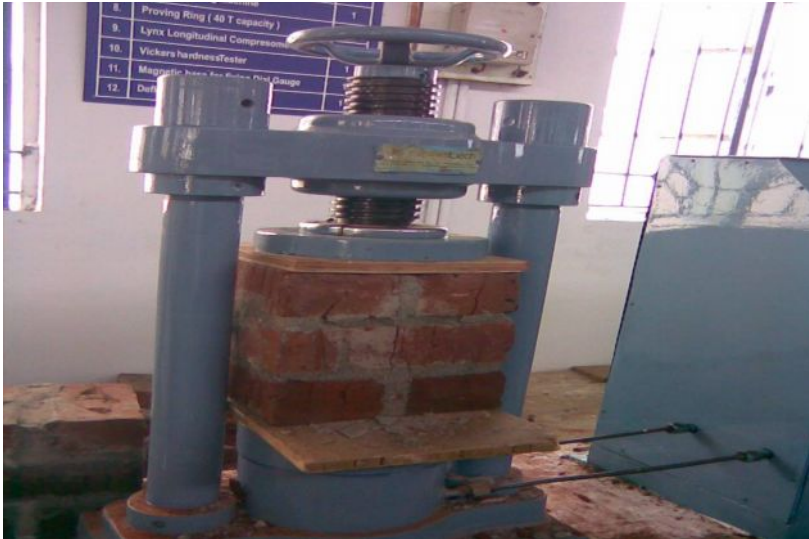
Fig 7 Photograph showing the test setup for brick prism compressive strength in compression testing machine
